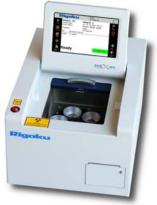
The Rigaku NEX QC is designed to be an ideal tool for reliably measuring the iron content in sand, and can be used at the quarry as well as along the production line to help ensure the highest quality while minimizing wastes and cost overruns.
